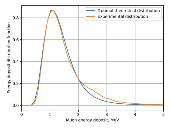
This new calibration method allows one to calibrate the detector channels via all muons registered, not only vertical muons.
